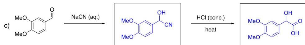
Similar to Q4 (b), however we are directly adding cyanide in the first step, therefore the first intermediate is the cyanohydrin. Hydrolysis of the cyanohydrin yields an  $\alpha$ -hydroxy acid.
