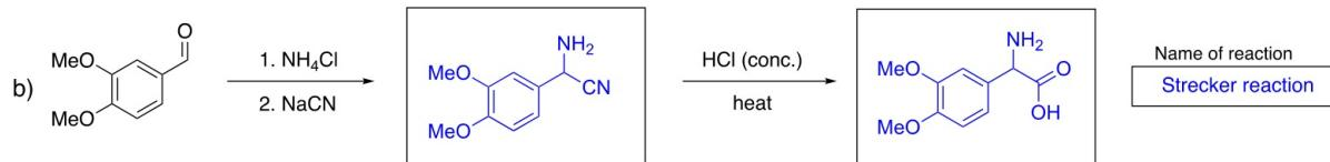
Typical Strecker synthesis conditions, formation of the imine (step 1) followed by addition of cyanide. Subsequent hydrolysis of the nitrile into a carboxylic acid furnishes the  $\alpha$ -amino acid.
